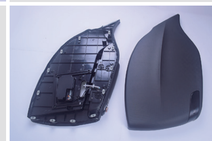
Here is how you detach the side board cover.
