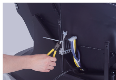
Here is the cable tie you are to cut off.
